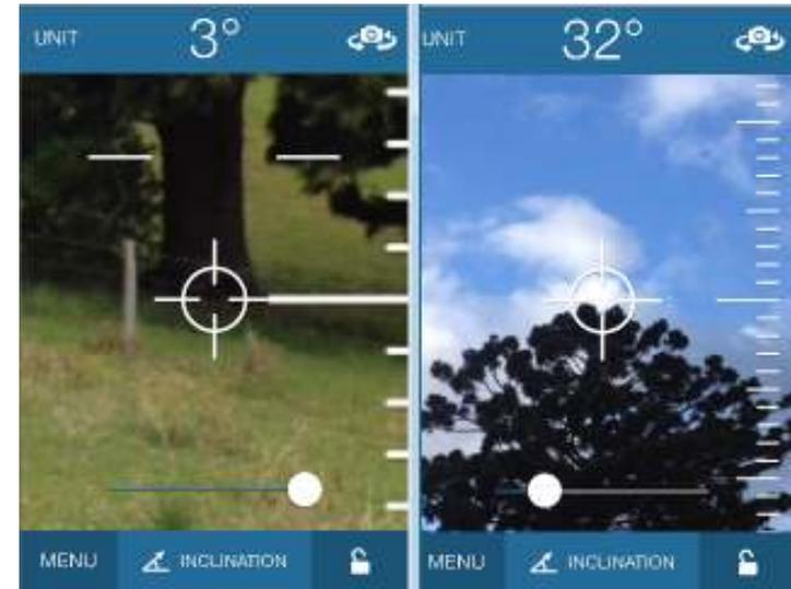
If instrument and reading errors on angles  $l_o$  &  $h_i$  are each  $\pm 1^\circ$ , then accuracy of height measure is  $\pm 5$  to  $6\%$  of height. eg  $\pm 1.5\text{m}$  on the  $\sim 30\text{m}$  tree illustrated here at  $40\text{m}$  distance.
